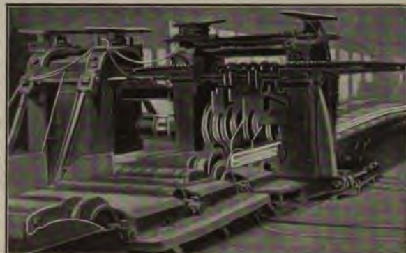
The steel ingot is heated again, rolled and cut into two or three lengths called blooms. The blooms are again heated and taken to the great-rail mill where they are rolled into steel rails. This cut shows one of the rolling mills.
